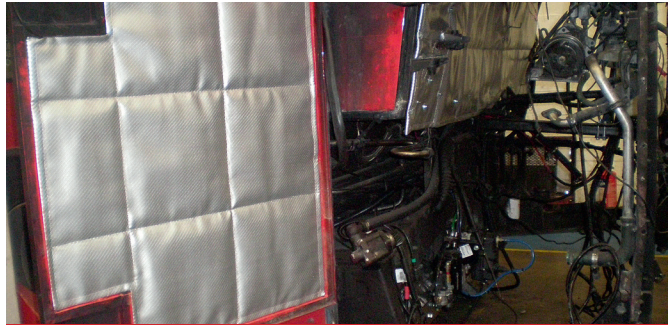
Bespoke eQuilt installed in modified Plaxton President being returned to use
