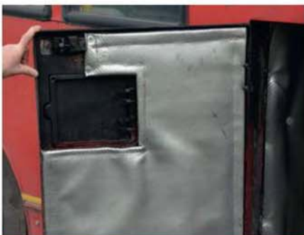
eQuilt looks like conventional sound insulation
