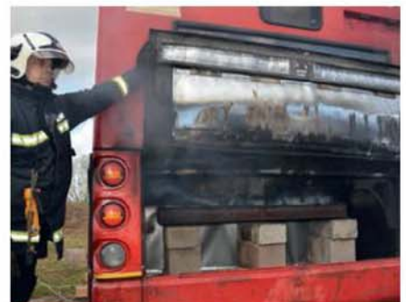
eQuilt expands 25 times during the fire
